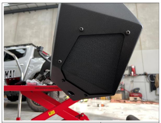
20. Fit plastic radar windows to the inside of the opening in the wing of the rear bar, using supplied M6x16 black bolts, flat washers, and flange nuts.
