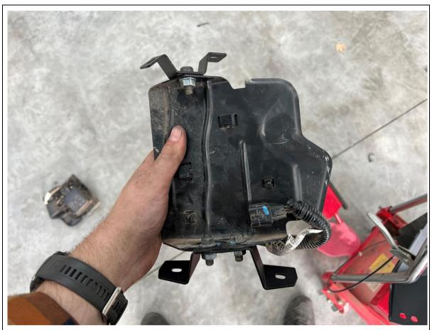
21. Fit the mounting brackets to the radar sensor bracket that contains the rear radar module.
