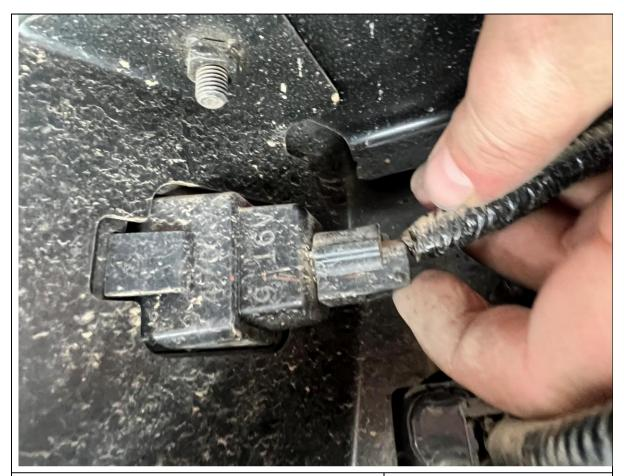
16. Disconnect the number plate light wiring connectors from the lamp housings.
